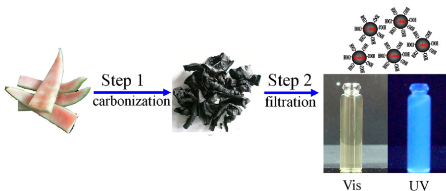
Scheme 1. Schematic illustration of the synthesis of water-soluble fluorescent C-dots from watermelon peel.
